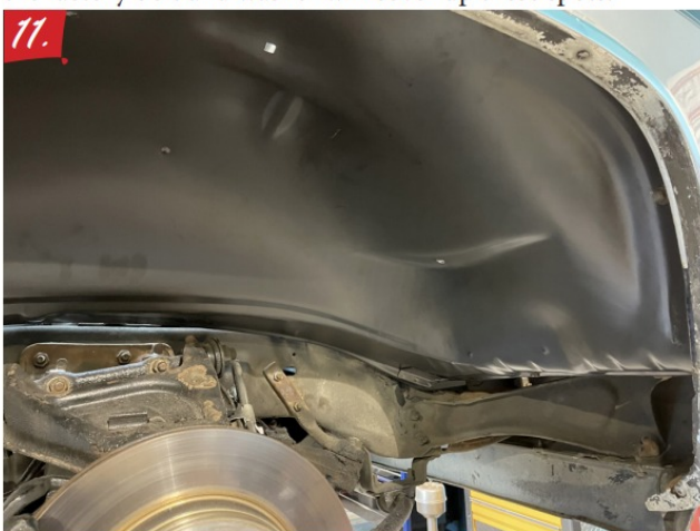
11. As you can see, the new early model inner fenders from AMD give you that extra tire clearance and maintain an original look
