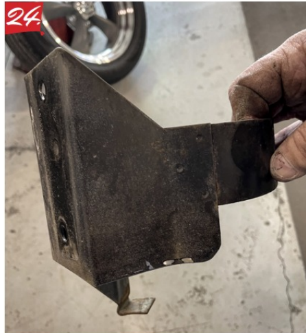
24. Using his cut off wheel, Harrison trims the bracket to remove any interference. Just enough to retain structural integrity
