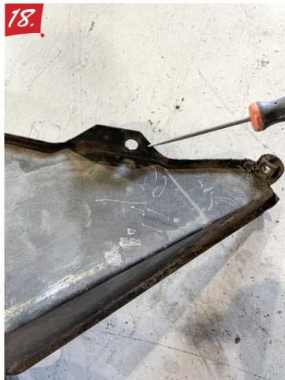
18. The center tab is drilled for mounting on the inner fender. This serves as a mockup to drill the inner fender for the 3/8-16 x 3/4" bolt.
