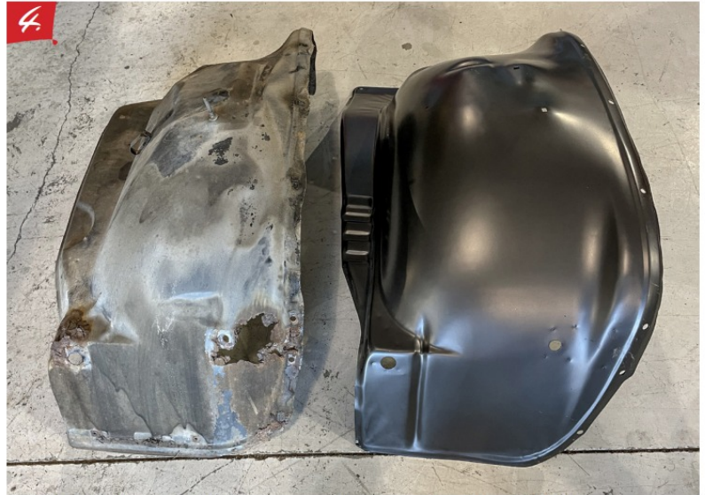
4. With the original inner out and next to the 73-80 AMD version, you can see just how much clearance you're going to gain over the factory 81-87 inner fender.
