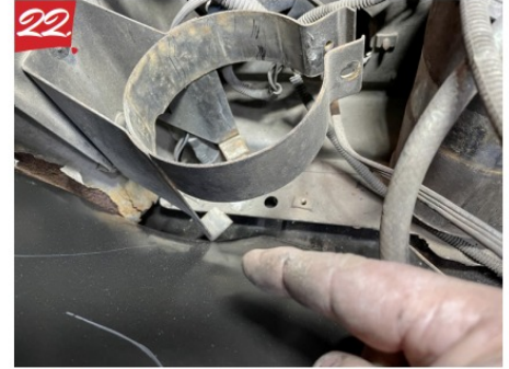
22. Moving to the driver side. The vapor canister needs some slight modifications as well.
