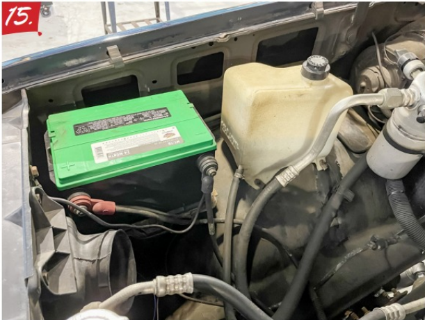
15. The other part of this conversion deals with modifying the battery tray and overflow canister.
