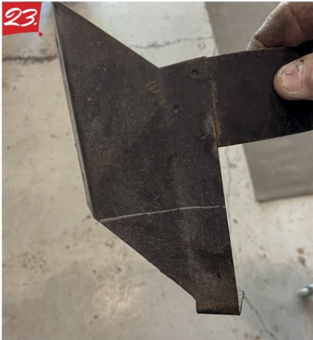
23. The canister bracket is marked to be cut as the early model inner fenders interfere with the lower foot on this bracket.
