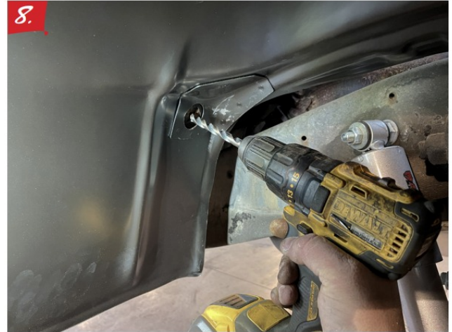
8. The same procedure is used for the inner brace as well. Patience is key, you don't want to go too far and damage the factory threads that you will be using.
