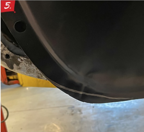
5. First mod, we need to trim the new inner fender to contour properly with the fender. You can use tin snips or your cut off wheel for this.
