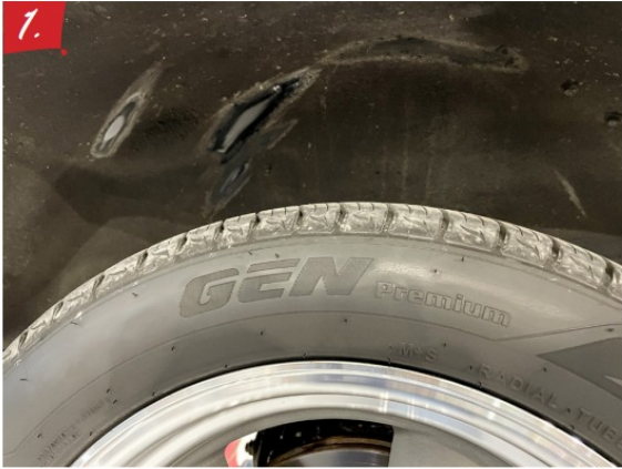
1. As you can tell, the 5inch drop on the front has some clearance issues when this truck hits a bump in the road.
