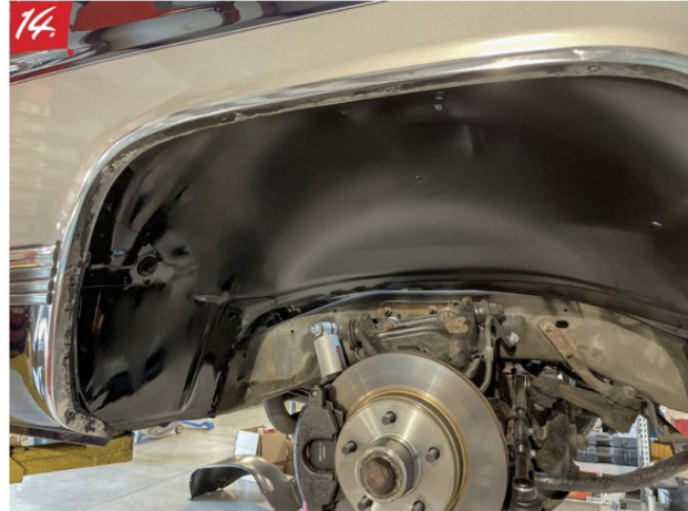
14. Harrison applies a light coat of sealer to finish off the installation underneath.
