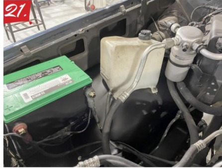
21. This truck came with a fender mounted overflow tank, Harrison re-mounts that by simply marking the holes, drilling the inner fender and uses the factory bolt and u-nut to remount the reservoir.
