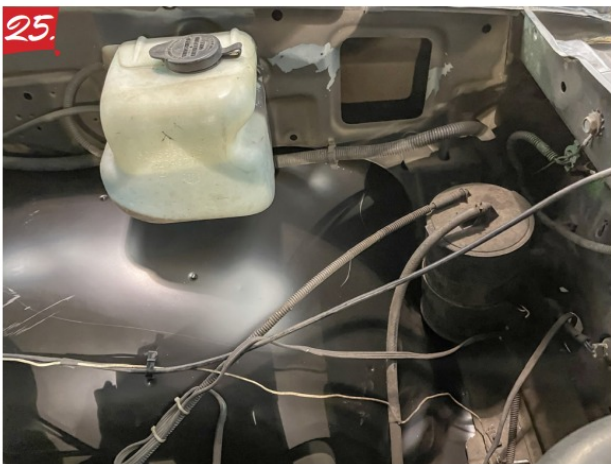
25. Drill holes as needed to remount the existing harness just like original.
