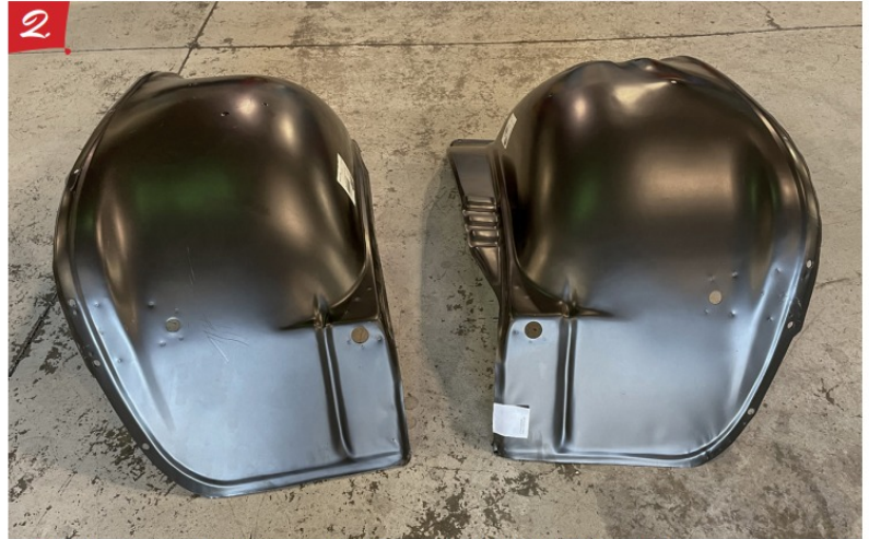
2. New inner fenders arrived from Auto Metal Direct, these work on all 73-80 GM Trucks, Blazers, Jimmys and Suburbans.
