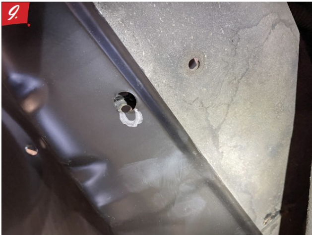
9. The holes at the front that connect to the core support need to be adjusted as well. Only slight adjustments are necessary, the factory bolt and washer will cover up these spots.
