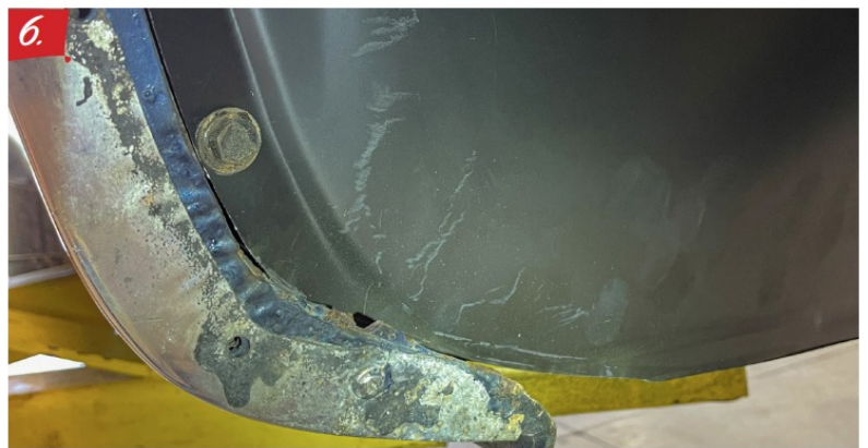
6. With the trimming done, you can see that the factory hole lines up, and you can start bolting it in
