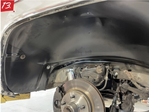
13. The same process is carried over to the driver side, all the original wheel arch bolts are reused as well.
